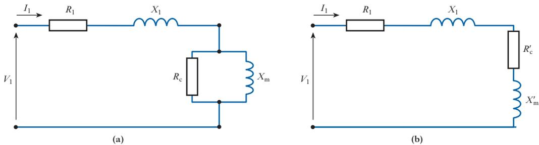
**Fig. 33.15** No-load equivalent circuits
