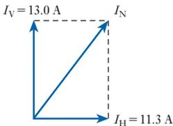
**Fig. 28.18** Vertical and horizontal components of  $I_N$
