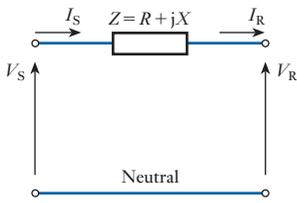
**Fig. 35.2** Equivalent circuit of short transmission line.  $V_S$  is the sending-end voltage,  $V_R$  is the receiving-end voltage
