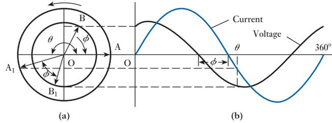
the voltage is represented by the projection of OB on the vertical axis. These values correspond to instant O in Fig. 9.17(b).
