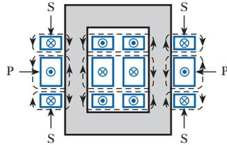
**Fig. 29.16** Shell-type construction
