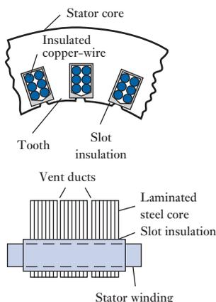
**Fig. 31.1** Portion of stator of a.c. synchronous machine
