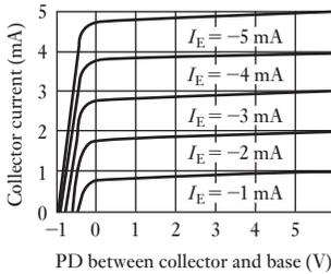
**Fig. 20.20** Static characteristics for a common-base n-p-n transistor circuit
