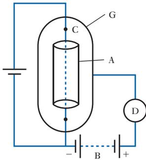
Fig. 42.2 A vacuum diode
