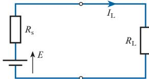
**Fig. 18.4** Energy source feeding load
