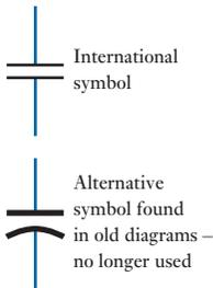
**Fig. 5.2** Circuit symbols for a capacitor
