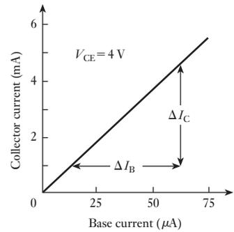
**Fig. 20.24** Relationship between collector and base currents, for a given collector-emitter voltage
