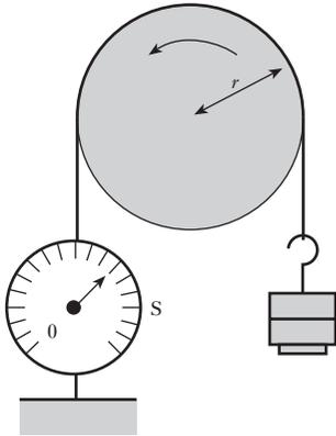
Fig. 39.11 Brake test on a motor
