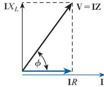
Fig. 12.7 Phasor diagram for  $R$  and  $L$  in series
