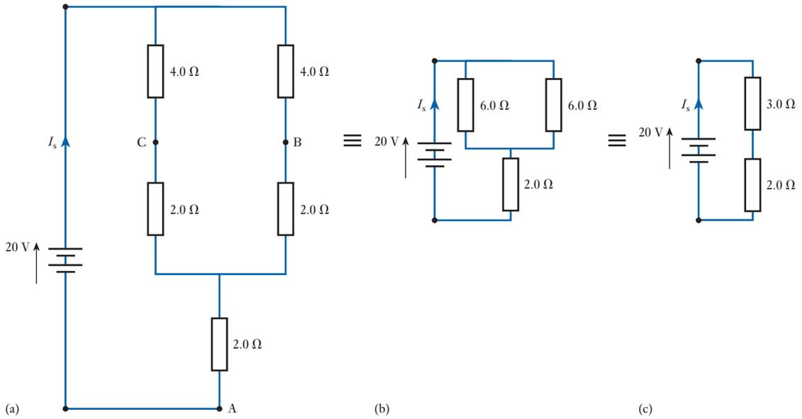
Fig. 4.42 T equivalent circuit reduction for Example 4.20
