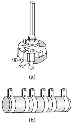
**Fig. 2.11** Variable resistors. (a) Wire-wound; (b) mains 'dropper' resistor with fixed tapings; cement coated on a ceramic former
