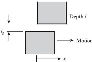
**Fig. 30.13** Lateral force between magnetized surfaces
