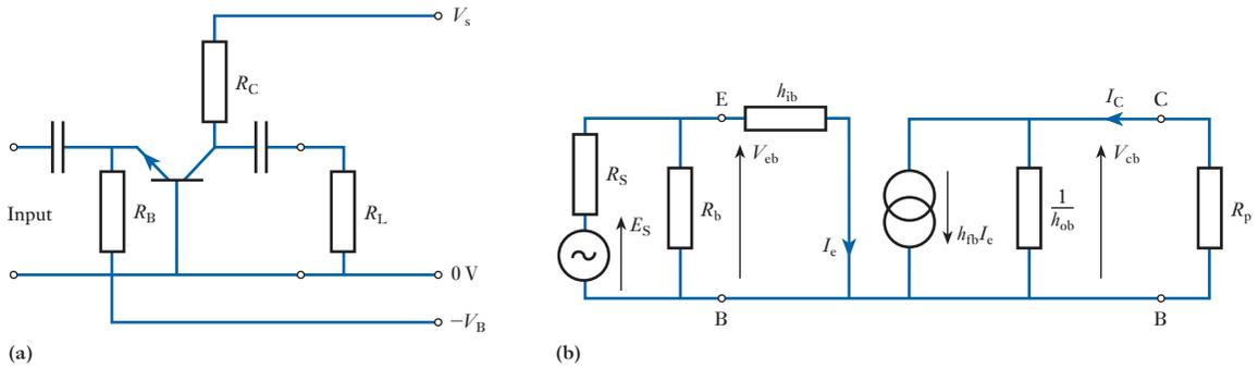
**Fig. 20.41** Common-base amplifier stage and its equivalent circuit
