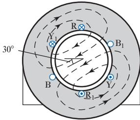
**Fig. 31.15** Distribution of magnetic flux at instant *b* of Fig. 31.11
