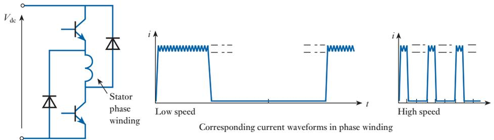
**Fig. 38.11** Drive circuit for a VR motor
