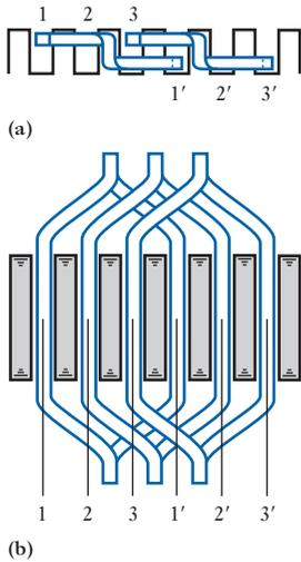
**Fig. 36.6** Arrangement of overlap of end connections
