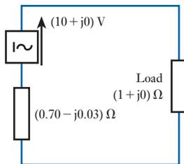
**Fig. 15.43** Equivalent circuit diagram for Example 15.17
