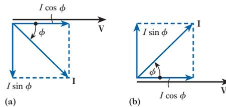
Consider Fig. 11.6 in which the current  $I$  is shown to lag (or lead) the voltage  $V$  by a phase angle  $\phi$ . This current may be made up by two components at right angles to one another:
