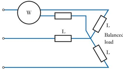
**(b) Balanced or unbalanced load, star- or delta-connected. The two-wattmeter method**
