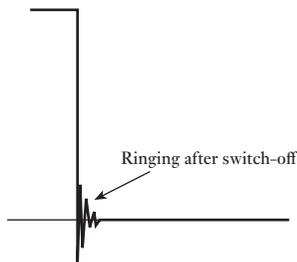
**Fig. 40.18** The ringing effect before snubbing
