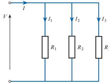
In this investigation, voltmeters are connected across each of the lamps while a further voltmeter is connected across the supply. Different supply voltages are applied to the network and it is observed that no matter what supply voltage is applied, the voltages across each of the loads are equal to it.
