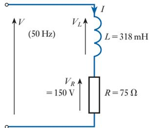
**Fig. 10.14** Circuit diagram for Example 10.2
