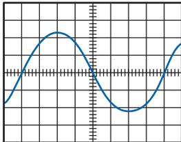
**Fig. 42.19** Sine waveform display on an oscilloscope
