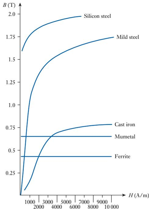
**Fig. 7.4**  $\mu_r/H$  characteristics for soft-magnetic materials
