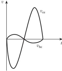
**Fig. 20.37** Common-emitter transistor input and output voltage waveforms
