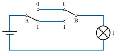
**Fig. 23.3** Switch arrangement equivalent to the EXCLUSIVE-OR logic
