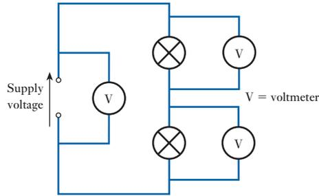
therefore the same, which is reasonable because where else can the current flow having passed through the first lamp but on through the second lamp, there being no other conduction path shown as available to the current?
