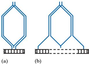
**Fig. 36.7** (a) Coil of a lap winding; (b) coil of a wave winding
