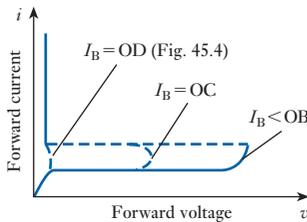
**Fig. 40.5** Variation of breakover voltage with bias current,  $I_B$
