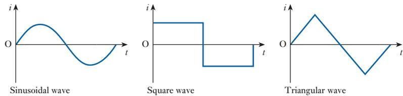
Alternating current can be abbreviated to a.c., hence a system with such an alternating current is known as an a.c. system. The curves relating current to time are known as *waveforms*. Those shown in Fig. 9.1 are simple waveforms, but waveforms can be quite complicated as shown in Fig. 9.5.
