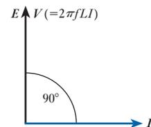
**Fig. 10.9** Phasor diagram for a purely inductive circuit
