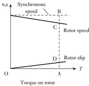
**Fig. 33.3** Slip and rotor speed of an induction motor
