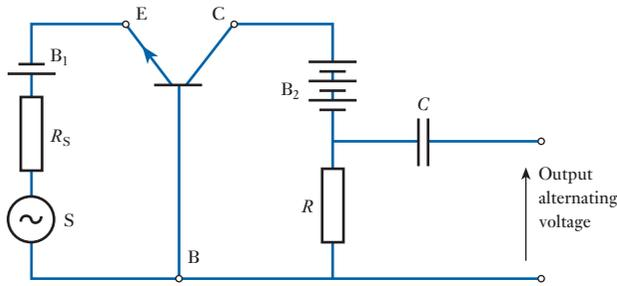
**Fig. 20.27** Graphical determination of the output current of a transistor in a common-base circuit
