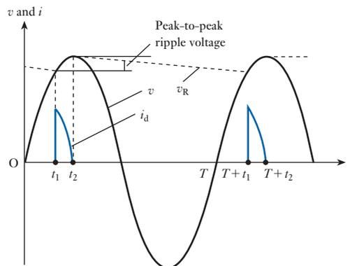
**Fig. 20.10** Waveforms for full-wave rectifier with capacitor input filter
