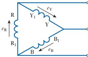
**Fig. 28.7** Conventional representation of a delta or mesh-connected winding
