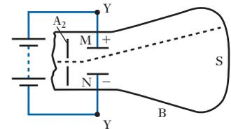
Fig. 42.14 Electrostatic deflection of an electron beam
