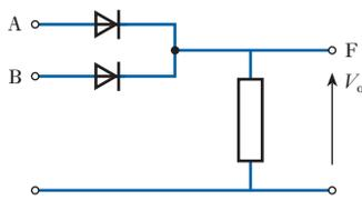
**Fig. 23.4** Simple OR gate circuit
