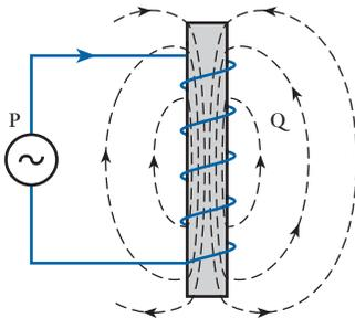
**Fig. 13.3** Magnetic field of an inductive circuit
