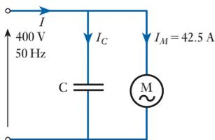
Fig. 13.11 Circuit diagram for Example 13.5
