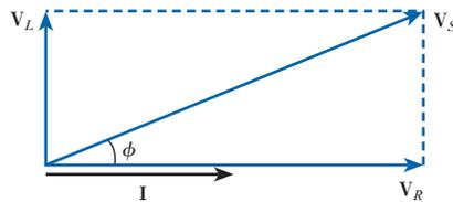
If each of the current phasors ( $I$ ,  $I \cos \phi$  and  $I \sin \phi$ ) is multiplied by the applied voltage  $V$ , then the *power triangle* is obtained, shown in Fig. 12.22.
