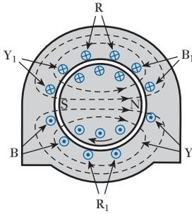
**Fig. 32.4** Resultant magnetic flux for case (b)
