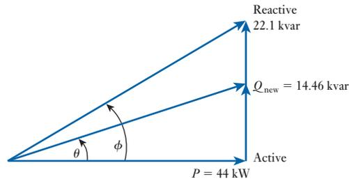
Also shown is the new value of power factor (0.95 lag), after the addition of capacitance. Capacitance must be added in order to correct to this new phase angle:
