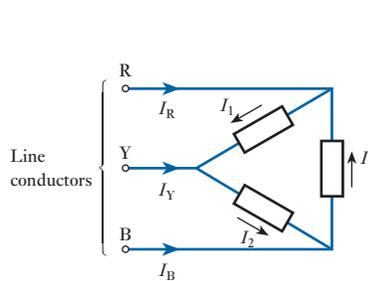
**Fig. 28.14** Delta-connected system with balanced load
