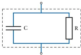
Fig. 5.32 Equivalent circuit of a practical capacitor
