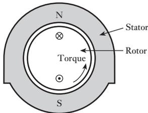
**Fig. 30.4** Rotary machine illustrating force of interaction
