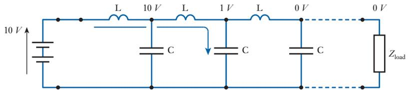
(D) The battery has charged the entire transmission line, and now current flows through the load.  $I = V_{\text{source}}/Z_{\text{load}}$
