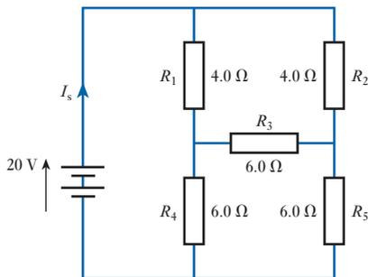
Resistors  $R_3$ ,  $R_4$  and  $R_5$  make up a  $\pi$  (or  $\Delta$ ) circuit. This is the part to be converted to a T (or Y) circuit. It is often the case with simple circuits that it is easier to calculate the new circuit element values from first principles, instead of applying equations [4.8] etc. It is certainly the case here. Since the elements of the  $\pi$  circuit are identical, so are those of the T equivalent circuit. In the  $\pi$  circuit of Fig. 4.41(a):
