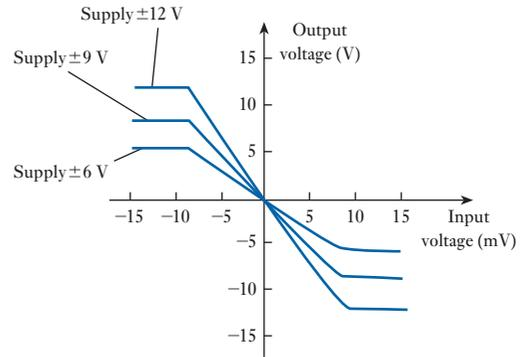
**Fig. 25.16** Forward characteristics of d.c. amplifier
