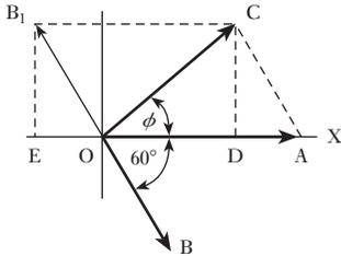
**Fig. 9.21** Subtraction of phasors for Example 9.7
