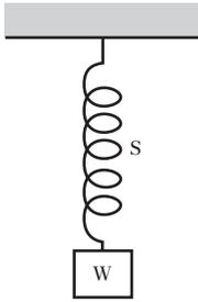
Fig. 14.12 Mechanical analogy of a resonant circuit
