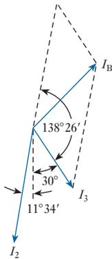
**Fig. 28.22** Phasor diagram for deriving  $I_B$
