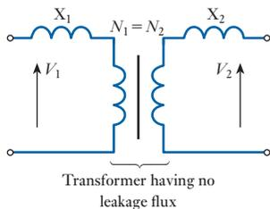
**Fig. 29.13** Transformer with leakage reactances
