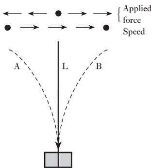
**Fig. 10.21** Mechanical analogy of a capacitive circuit
