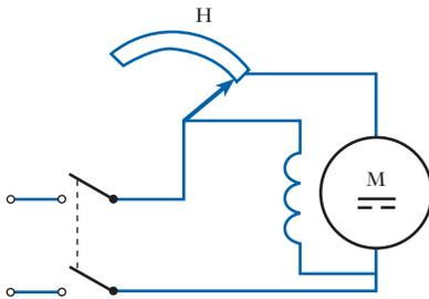
Fig. 37.4 Shunt-wound motor
