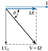
Fig. 12.8 Phasor diagram for  $R$  and  $C$  in series
