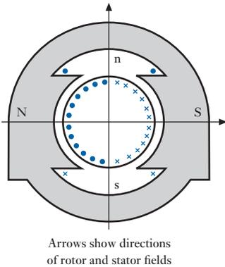
Arrows show directions of rotor and stator fields
