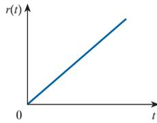
**Fig. 24.8** The unit ramp function
