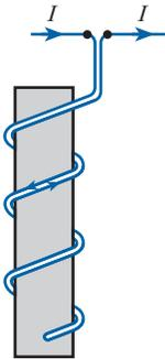
Fig. 8.3 Non-inductive resistor
