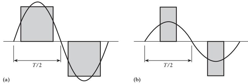
**Fig. 40.17** PWM voltage control
