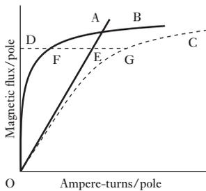
Fig. 37.2 Magnetization curve of a machine
