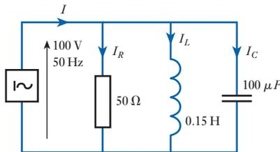
(a) The circuit diagram is given in Fig. 11.4, where  $I_R$ ,  $I_L$  and  $I_C$  represent the currents through the resistance, inductance and capacitance respectively.
