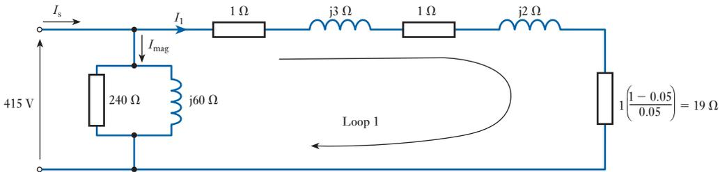
**Fig. 33.10** Equivalent circuit for Example 33.4
