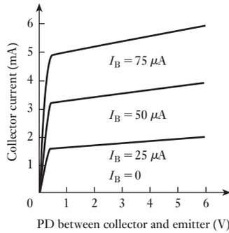
**Fig. 20.23** Static characteristics for a common-emitter n-p-n transistor circuit
