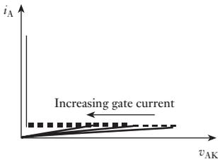
**Fig. 40.9** Forward conduction characteristic of thyristor
