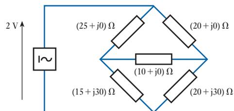
**Fig. 15.23** Circuit diagram for Example 15.12
