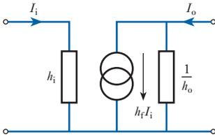
**Fig. 20.35**  $h$ -parameters for a transistor equivalent circuit
