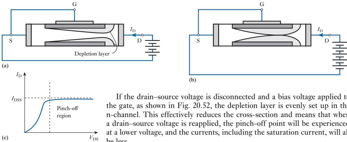
**Fig. 20.51** Depletion layer in a JUGFET
