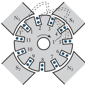
**Fig. 36.4** Arrangement of a double-layer winding
