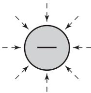
**Fig. 5.9** Electric field about an isolated spherical charge
