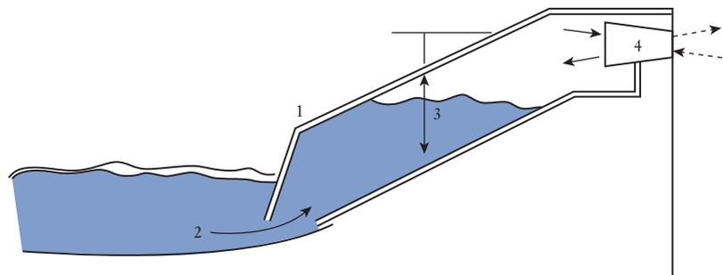
1. Wave capture chamber set into rock face
