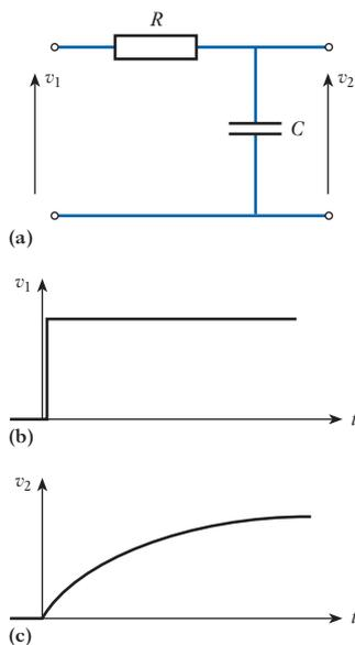
**Fig. 41.8** Signal transfer in an  $RC$  network
