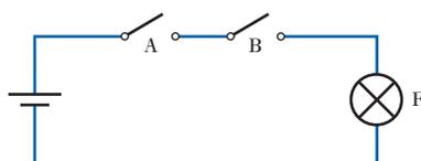
**Fig. 23.2** Switch arrangement equivalent to AND logic**Table 23.2**
