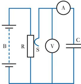
**Fig. 5.16** Charging and discharging of a capacitor
