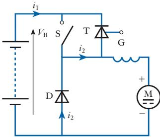
**Fig. 37.11** Chopper speed control of a series motor
