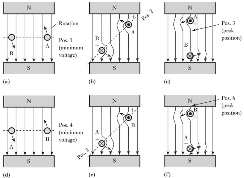
a coil side. Once the coil reaches the position shown in Fig. 9.3(c), the rate of cutting reaches a maximum. Thereafter the e.m.f. falls to zero by the time the coil has rotated to the position shown in Fig. 9.3(d).
