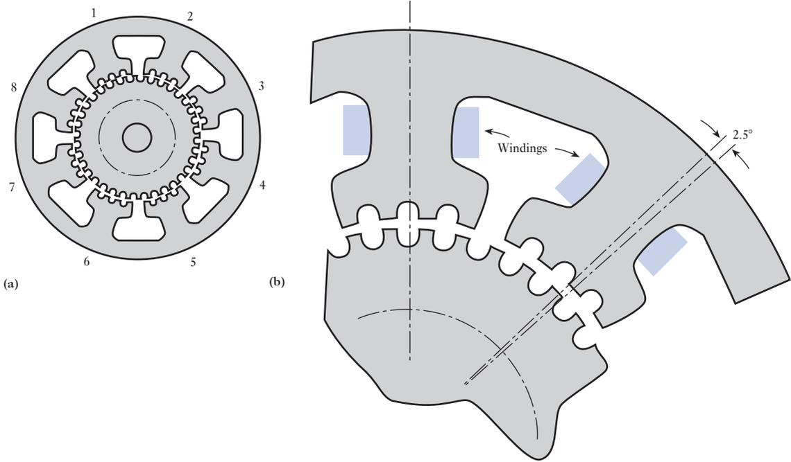
**Fig. 38.8** Construction of a hybrid stepping motor (144 steps per revolution)
