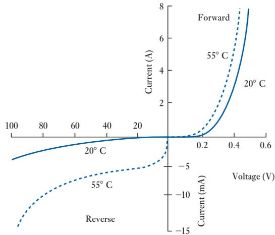
**Fig. 19.18** Static characteristics of a silicon junction diode
