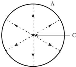
Fig. 42.3 Electron paths from cathode to anode
