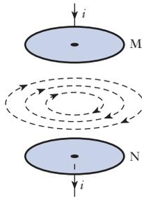
**Fig. 5.34** Magnetic field due to displacement current
