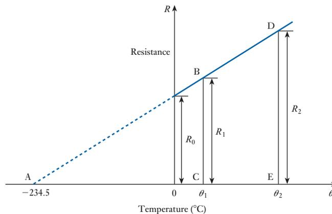
axis is found to be  $-234.5^{\circ}\text{C}$ . Hence, for a copper conductor having a resistance of  $1\ \Omega$  at  $0^{\circ}\text{C}$ , the change of resistance for  $1^{\circ}\text{C}$  change of temperature is  $(1/234.5)\ \Omega$ , namely  $0.004\ 264\ \Omega$ ,
