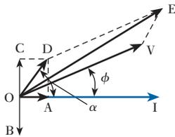
**Fig. 32.8** Phasor diagram for a synchronous generator
