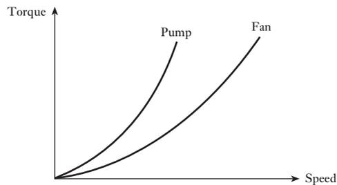
**Fig. 39.5** Motor and load torque characteristics for a fan
