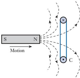
**Fig. 6.20** Distortion of magnetic field by induced current
