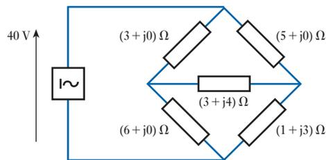
**Fig. 15.9** Circuit diagram for Example 15.6
