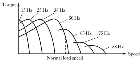
**Fig. 40.27** Inverter-fed variable-frequency induction motor
