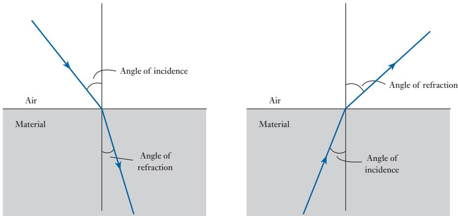
**Fig. 27.3** Light refraction
