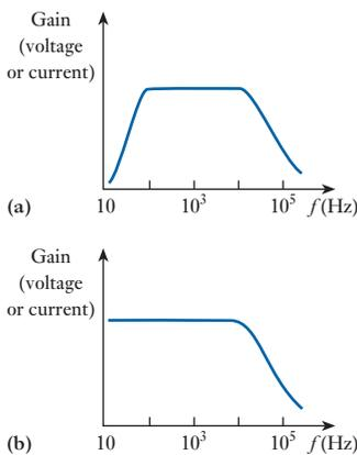
**Fig. 25.14** Gain/frequency characteristics.
