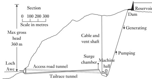
Figure 34.9 shows details of the Cruachan pump-storage station in Scotland. It has four 100 MW machines which can operate both as pumps and as generators. They can be run up to full generating capacity in 30 seconds. The scheme has an overall energy efficiency of about 80 per cent. However, as electricity is used in the pumping process, pumped storage stations are net consumers of electricity.
