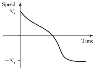
**Fig. 33.22** Speed/time characteristic of a plugging motor
