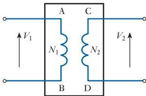
**Fig. 29.12** Ideal transformer enclosed in a box
