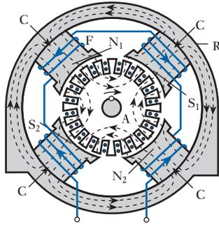
Fig. 36.1 General arrangement of a four-pole d.c. machine
