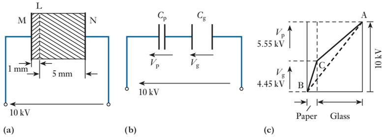
(a) Figure 5.15(a) shows a cross-section (not to scale) of the capacitor; and in Fig. 5.15(b),  $C_p$  represents the capacitance of the paper layer between M and the equipotential surface L and  $C_g$  represents that of the glass between L and N. From expression [5.13] we have
