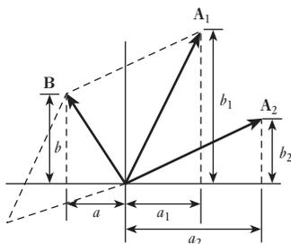
**Fig. 12.6** Subtraction of phasors
