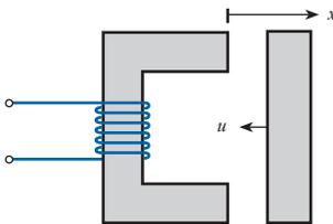
Fig. 30.11 Attracted-armature relay operation
