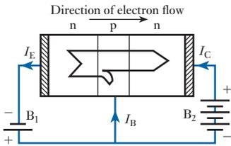
**Fig. 20.14** Electron flow in an n-p-n transistor
