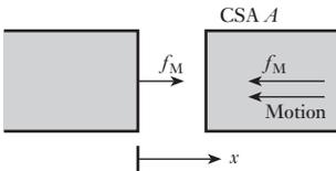
**Fig. 30.12** Force of alignment between parallel magnetized surfaces
