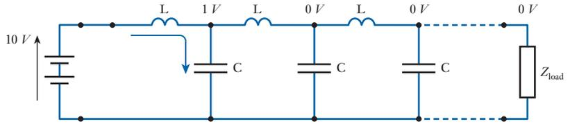
(C) The battery has charged up the first stage and is now charging the second stage. The current  $I = V_{\text{source}}/Z_0$
