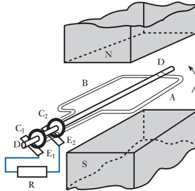
**Fig. 9.3** EMF in rotating coil
