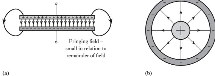
It should not be overlooked that the space between the conductors needs to be filled with an insulator, otherwise the charges would move towards one another and therefore be dissipated. The insulant is called a dielectric.
