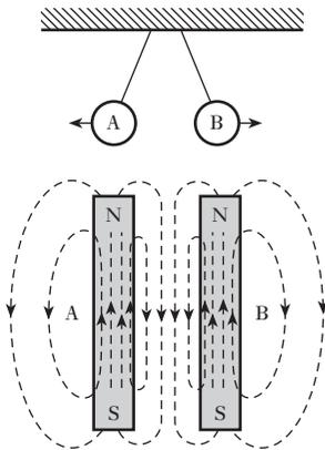
**Fig. 6.5** Repulsion between magnets
