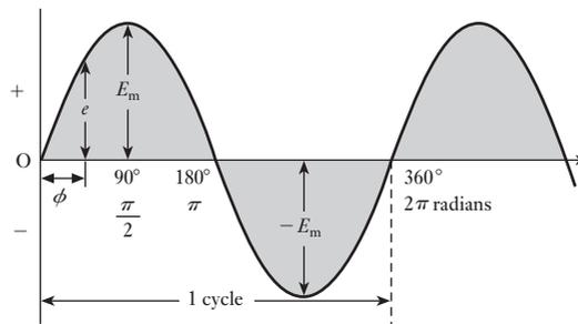
Fig. 9.6 Extended sine wave of e.m.f.
