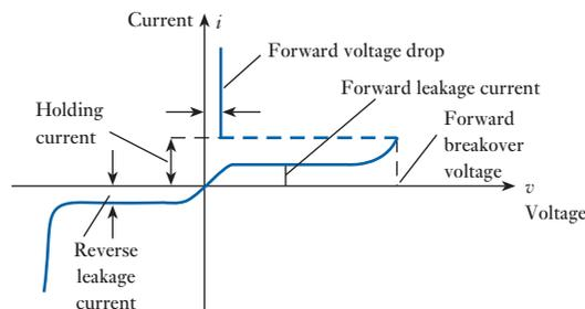
**Fig. 40.3** Gate control of thyristor breakover voltage
