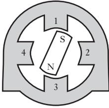
Fig. 38.5 Simple stepping motor
