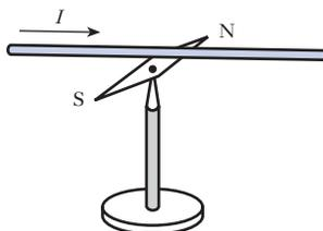
**Fig. 6.6** Oersted's experiment
