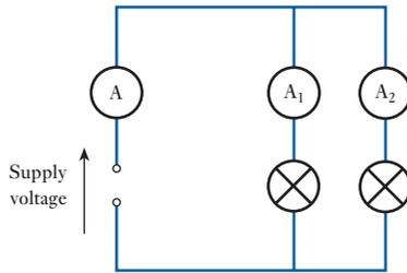
It may be observed that no matter what supply voltage is applied, the sum of the currents as indicated by ammeter A<sub>1</sub> and ammeter A<sub>2</sub> is always equal to the supply current as indicated by ammeter A. It makes no difference whether identical or dissimilar lamps are used – the results are always the same and
