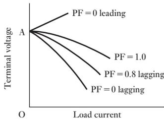
**Fig. 32.5** Variation of terminal voltage with load
