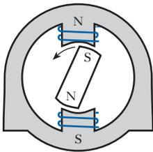
Fig. 38.4 Reluctance motor with permanent magnet rotor
