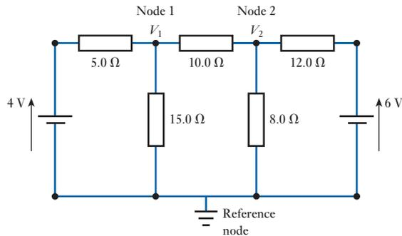
Step 1 Reference node shown. Voltages  $V_1$  and  $V_2$  assigned.
