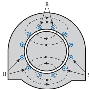
Fig. 32.2 Magnetic flux due to stator currents alone
