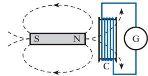
Fig. 6.17 Electromagnetic induction
