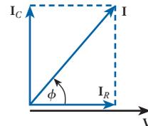
Fig. 12.14 Phasor diagram for Fig. 12.13
