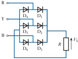
**Fig. 40.23** Three-phase bridge rectifier network
