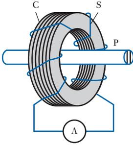
**Fig. 29.27** A bar-primary current transformer
