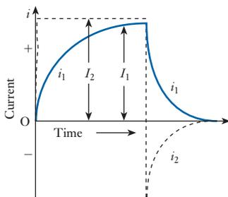
**Fig. 8.2** Variation of switch-on and switch-off currents
