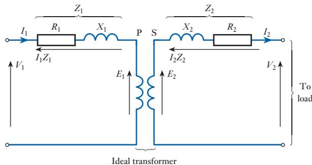
**29.13** Simplification of the approximate equivalent circuit of a transformer
