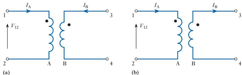
and the mutual inductance is then said to be *positive*. But if  $I_A$  enters coil A at the dotted end and  $I_B$  leaves coil B at the dotted end, as in Fig. 8.24(b), the m.m.f.s of the coils are in opposition and the mutual inductance is then said to be *negative*.
