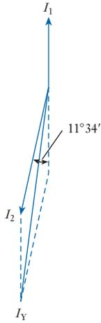
**Fig. 28.21** Phasor diagram for deriving  $I_Y$
