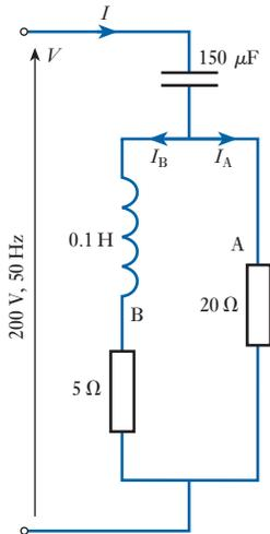
**Fig. 12.17** Circuit diagram for Example 12.5
