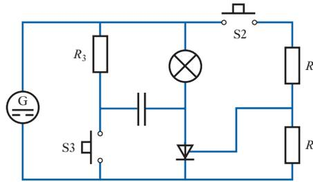
**Fig.40.8** Simple d.c. thyristor on-off circuit
