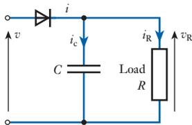
**Fig. 20.8** Half-wave rectifier with capacitor input filter
