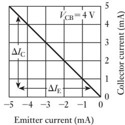
**Fig. 20.21** Relationship between collector and emitter currents for a given collector-base voltage
