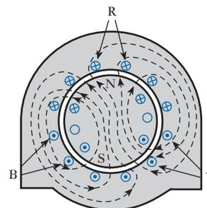
Fig. 32.3 Resultant magnetic flux for case (a)
