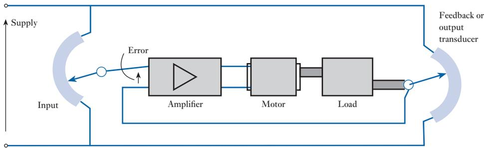
**Fig. 41.11** Simple servomechanism or r.p.c.
