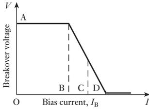
**Fig. 40.4** Variation of breakover voltage with bias current
