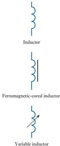
**Fig. 8.23** Circuit symbols for inductors
