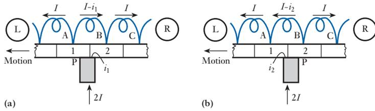
**Fig. 36.14** Variation of current in the short-circuited coil
