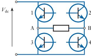
**Fig. 40.14** Inverter network for one-phase supply
