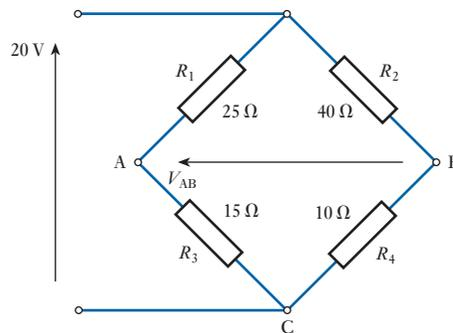
The rearrangement of the drawing layout of a network sometimes gives rise to confusion, and it is worth noting that the network used in this example is often drawn in the form shown in Fig. 3.34. This form of circuit diagram is called a bridge.
