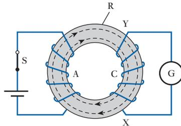
Fig. 6.16 Electromagnetic induction
