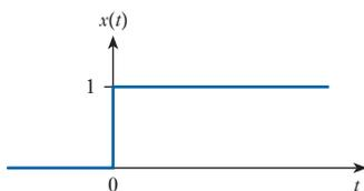
**Fig. 24.6** The unit step function
