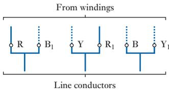
**Fig. 31.8** Delta connection of windings
