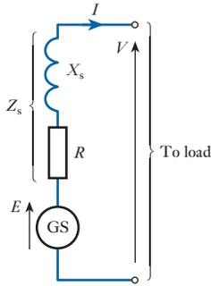
**Fig. 32.7** Equivalent circuit of a synchronous generator
