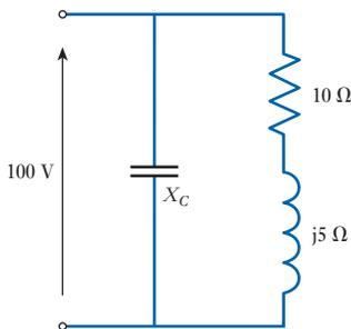
Fig. 13.13 Circuit for Example 13.7(a)
