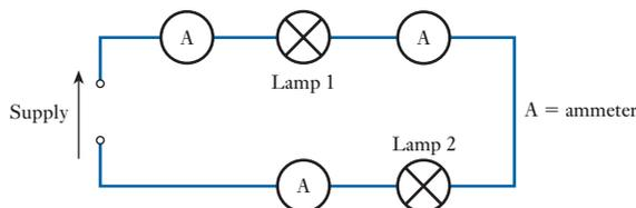
**Fig. 3.4** Investigation of volt drops in a series circuit
