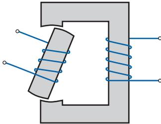
Fig. 30.19 Simple doubly excited rotary system
