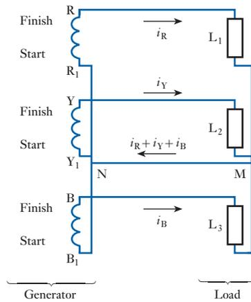
**Fig. 28.9** Four-wire star-connected system
