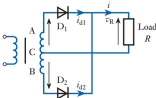
**Fig. 20.4** Full-wave rectifier with resistive load
