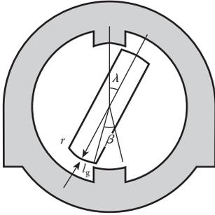
Fig. 30.17 Simple reluctance torque machine
