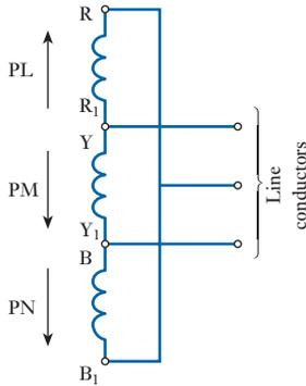
**Fig. 28.6** Delta connection of three-phase winding
