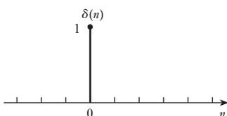
**Fig. 24.11** The discrete-time unit impulse
