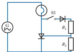
**Fig. 40.10** Simple half-wave a.c. switch circuit
