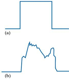
**Fig. 25.3** A transmitted pulse. (a) Input transmitted; (b) output received
