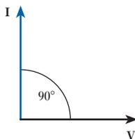
**Fig. 10.19** Phasor diagram for a purely capacitive circuit
