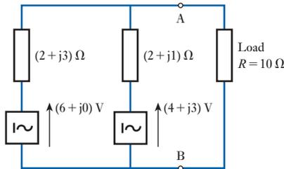
**Fig. 15.17** Circuit diagram for Example 15.10
