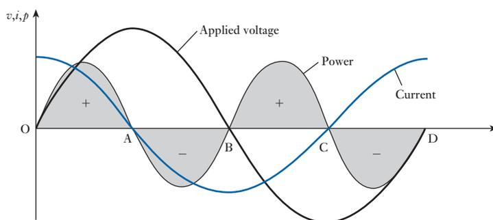
During interval AB, the p.d. across the capacitor decreases from its maximum value to zero and the whole of the energy stored in the capacitor at instant A is returned to the generator; consequently, the net energy absorbed during the half-cycle OB is zero. Similarly, the energy absorbed by the capacitor during interval BC is returned to the generator during interval CD. Hence the average power over a complete cycle is zero.
