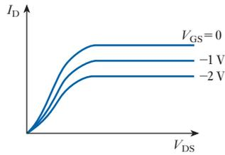
**Fig. 20.54** Output characteristics of an n-channel JUGFET
