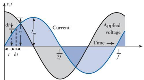
Hence the induced e.m.f. is represented by the curve in Fig. 10.7, leading the current by a quarter of a cycle.
