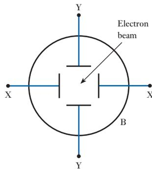
Fig. 42.13 Deflecting plates of a cathode-ray tube
