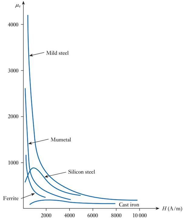
**Fig. 7.5**  $\mu_r/B$  characteristics for soft-magnetic materials
