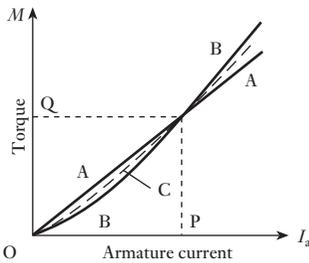
**Fig. 37.8** Torque characteristics of shunt, series and compound motors
