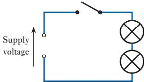
**Fig. 3.2** Incorrect lamp connection
