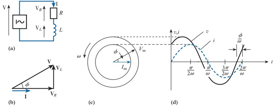
The phasor diagram results from an application of Kirchhoff's second law. For convenience, the current is taken as reference since it is common to all the elements of a series circuit. The circuit voltage may then be derived from the following relations:
