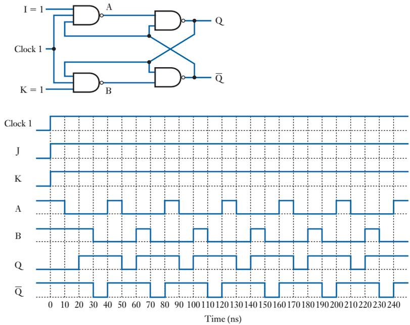
**Fig. 23.41** Master–slave JK flip-flop circuit
