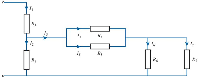
Starting with the points that may be readily observed, it can be seen that  $R_4$  is in parallel with  $R_5$ . Also  $R_6$  is in parallel with  $R_7$ . In each case the current divides between the two components and then comes together again.
