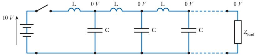
(B) The switch is closed. Current flows and the first C begins to charge. As it does, the voltage rises and current begins to flow to the second stage. The current  $I = V_{\text{source}}/Z_0$  where  $Z_0 = \sqrt{L/C}$
