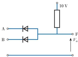
**Fig. 23.5** Simple AND gate circuit
