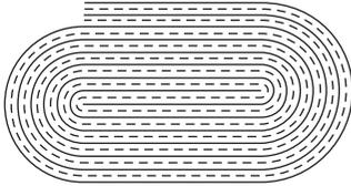
**Fig. 5.1** Paper-insulated capacitor
