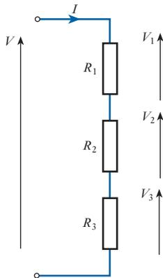
**Fig. 3.5** Volt drops in a series circuit
