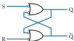
Fig. 23.37 Alternative SR circuit
