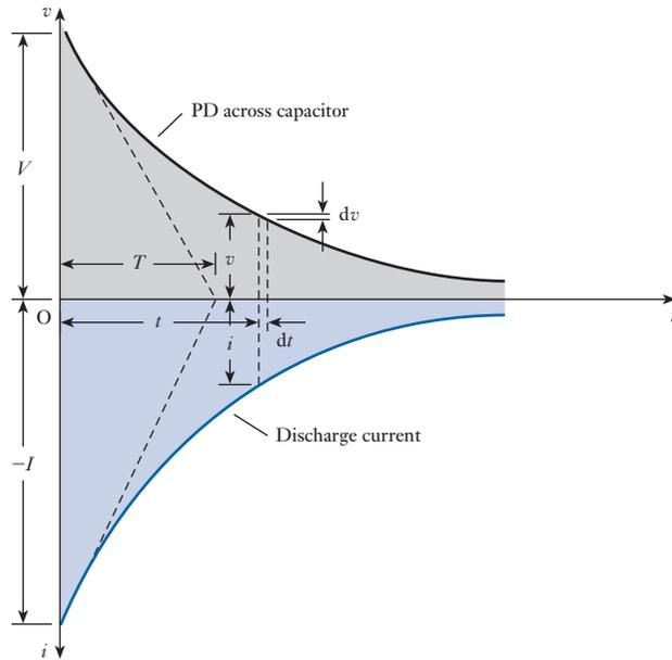
Suppose the p.d. across  $C$  to be  $v$  volts  $t$  seconds after  $S$  has been moved to position  $b$ , and the corresponding current to be  $i$  amperes, as in Fig. 5.22, then
