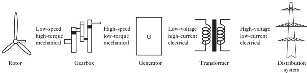
Fig. 34.11 Energy conversion in a wind turbine
