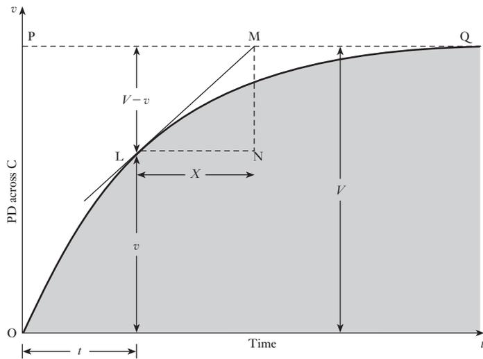
**Fig. 5.19** Growth of p.d. across a capacitor in series with a resistor
