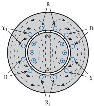
Fig. 32.1 Magnetic flux due to rotor current alone
