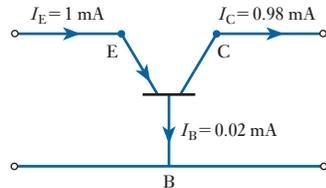
**Fig. 20.15** Currents in emitter, collector and base circuits of a p-n-p transistor
