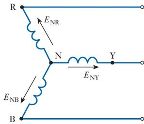
**Fig. 28.12** Star-connected generator
