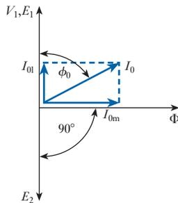
**Fig. 29.4** Phasor diagram for transformer on no load
