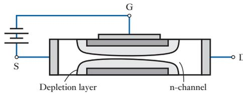
**Fig. 20.53** Combined depletion effects in a JUGFET
