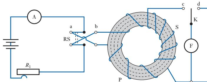
a certain value in one direction to the same value in the reverse direction. During this operation, switch K should be on d, thereby short-circuiting the fluxmeter. With switch RS on, say, a, switch K is moved over to c, the current through P is reversed by moving RS quickly over to b and the fluxmeter deflection is noted.
