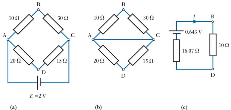
B being positive relative to D. Consequently, current in the  $40\ \Omega$  resistor, when connected between B and D, will flow from B to D.
