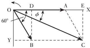
Fig. 9.20 Addition of phasors for Example 9.7
