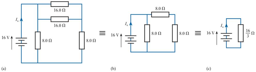
Fig. 4.45  $\pi$  equivalent circuit reduction for Example 4.21
