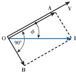
**Fig. 13.10** Active and reactive components of current
