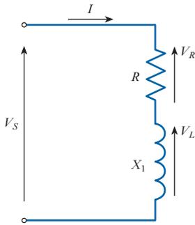
Fig. 12.20 Series RL circuit
