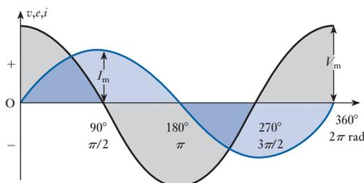
voltage applied to a purely inductive circuit leads the current by a quarter of a cycle or  $90^\circ$ , or the current lags the applied voltage by a quarter of a cycle or  $90^\circ$ .
