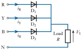
Fig. 40.21 Simple three-phase rectifier network
