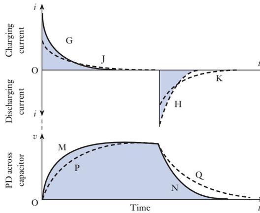
it takes about twice as long to rise up and to fall off, as shown by the dotted curves J and K. Curves P and Q represent the corresponding variation of the p.d. across C during charge and discharge respectively.
