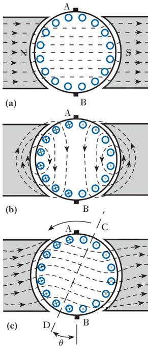
**Fig. 36.9** Flux distribution due to (a) field current alone, (b) armature current alone, (c) field and armature currents of a d.c. motor
