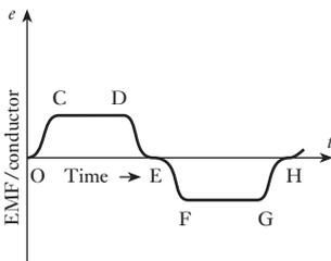
Fig. 36.2 Waveform of e.m.f. generated in a conductor
