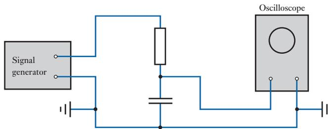
**Fig. 42.22** Unsuitable reconnection of the oscilloscope
