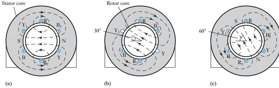
**Fig. 31.10** Distribution of magnetic flux due to three-phase currents
