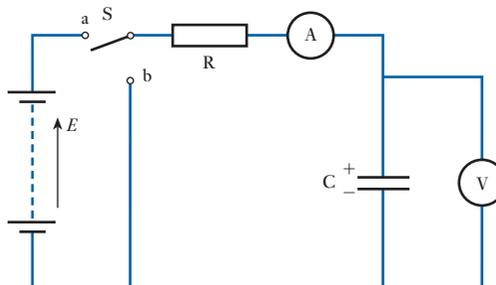
**Fig. 5.4** Charging and discharging currents and p.d.s
