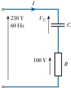
**Fig. 10.29** Circuit diagram for Example 10.7
