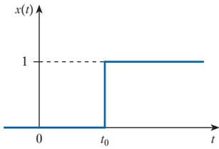
**Fig. 24.7** The delayed unit step function
