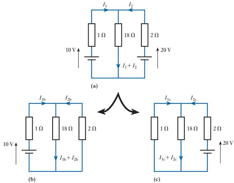
Because there are two sources of e.m.f. in the network, then two separate networks need to be considered, each having one source of e.m.f. Figure 4.20(b) shows the network with the 20 V source replaced by a short-circuit, there being zero internal resistance indicated. Also, Fig. 4.20(c) shows the network with the 10 V source similarly replaced.
