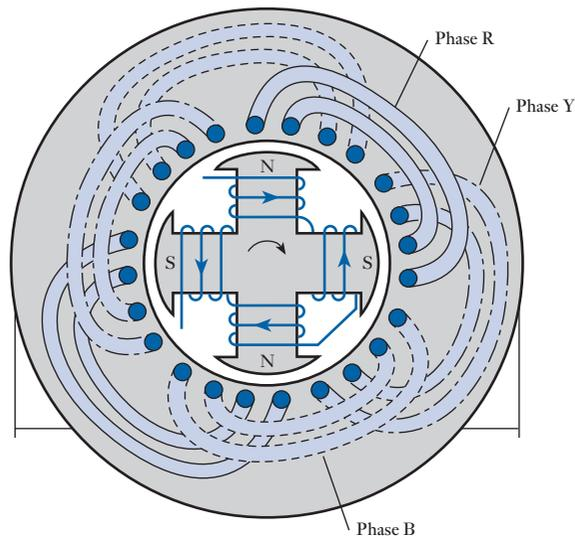
**Fig. 31.5** End connections of a three-phase single-layer winding
