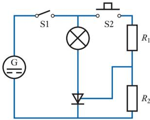
**Fig. 40.7** Simple d.c. thyristor switch-on circuit
