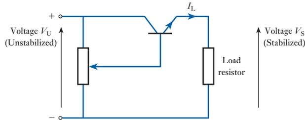
**Fig. 20.47** Stabilization circuit incorporating a comparator network
