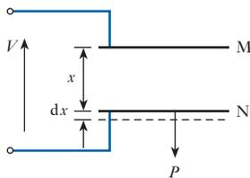
**Fig. 5.31** Attraction between charged parallel plates
