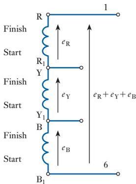
**Fig. 28.5** Resultant e.m.f. in a delta-connected winding
