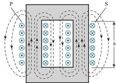
**Fig. 29.11** Paths of leakage flux
