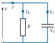
Fig. 12.13 R and C in parallel
