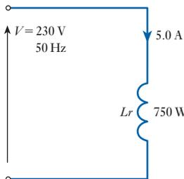
Fig. 13.9 Circuit diagram for Example 13.3
