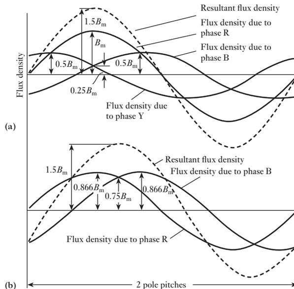
**Fig. 31.13** Distribution of flux densities due to three-phase currents
