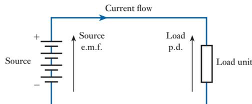
line as if it were a dimension line. An arrowhead is drawn on the transmission system to indicate the corresponding direction of conventional current flow.
