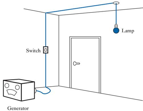
Fig. 2.3 Simple lamp circuit
