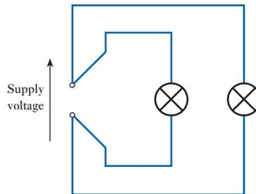
**Fig. 3.13** Correct lamp connection
