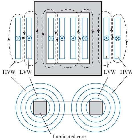
**Fig. 29.15** Sandwiched windings
