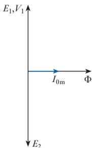
**Fig. 29.8** Phasor diagram for Fig. 29.7
