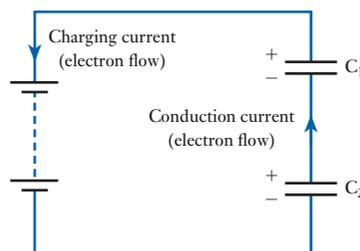
causes electrons to flow from the positive plate of  $C_1$  via the battery to the negative plate of  $C_2$ .
