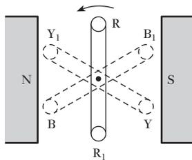
**Fig. 28.1** Generation of three-phase e.m.f.s
