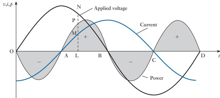
By repeating this calculation at various instants we can deduce the curve representing the variation of power over one cycle. It is seen that during interval  $OA$  the applied voltage is positive, but the current is negative, so that the power is negative; and that during interval  $AB$ , both the current and the voltage are positive, so that the power is positive.
