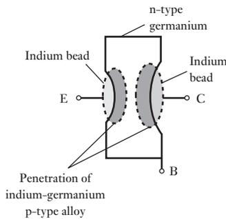
**Fig. 20.16** Construction of a p-n-p germanium transistor
