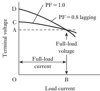
**Fig. 32.6** Variation of terminal voltage with load
