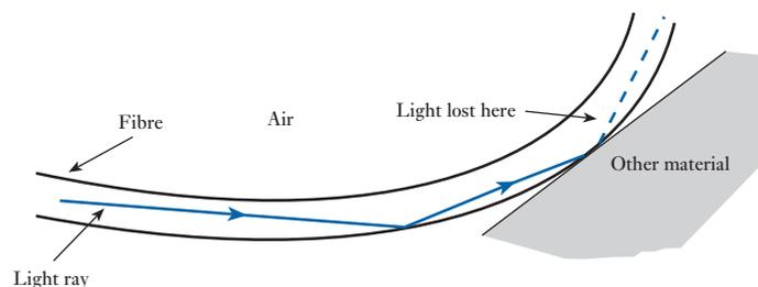
Fig. 27.2 Clad optical fibre
