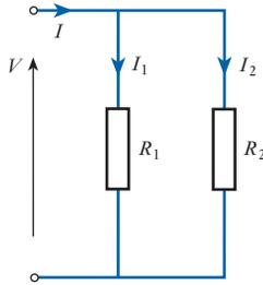
**Fig. 3.21** Circuit with two resistors in parallel
