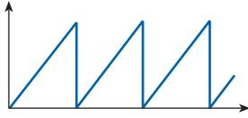
**Fig. 42.17** X-amplifier sawtooth waveform.
