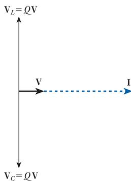
**Fig. 14.9** Voltage magnification  $Q$  in series resonant circuit
