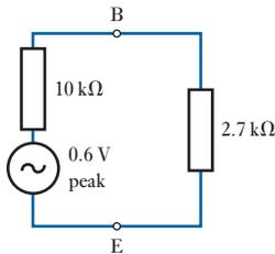
**Fig. 20.34** Equivalent input circuit for Example 20.3
