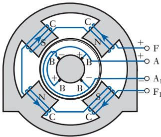
Fig. 37.1 Armature and field connections
