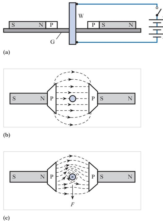
shown in Fig. 6.13(b). If the switch is closed momentarily, the filings rearrange themselves as in Fig. 6.13(c). It will be seen that the lines of magnetic flux have been so distorted that they partially surround the wire. This distorted flux acts like stretched elastic cords bent out of the straight; the lines of flux try to return to the shortest paths between PP, thereby exerting a force  $F$  urging the conductor out of the way.
