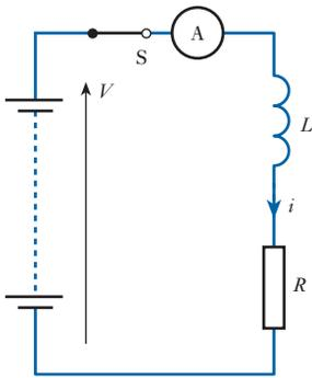
**Fig. 8.8** Inductive circuit
