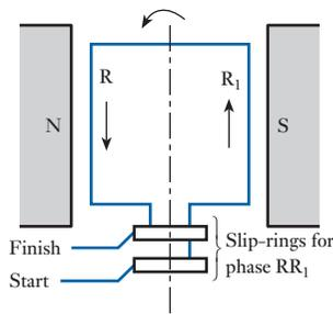
**Fig. 28.2** Loop RR<sub>1</sub> at instant of maximum e.m.f.
