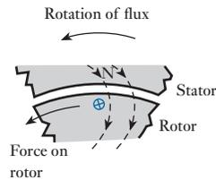
**Fig. 33.2** Force on rotor
