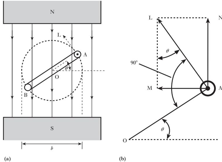
$AL$  drawn at right angles to the plane of the loop. We can resolve  $AL$  into two components,  $AM$  and  $AN$ , perpendicular and parallel respectively to the direction of the magnetic flux, as shown in Fig. 9.4(b). Since
